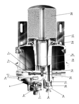
The Haldex Air Dryer is a desiccant type dryer that effectively removes moisture, oil and contaminants from the compressed air system. This reduces the risk of freezing or corrosion of the components in the air system. When compressor cut-out is reached, dry air is allowed to flow back to regenerate the desiccant bed.
