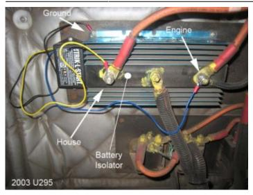
There are several devices that allow this on the market. One of the most popular is Trik-L-Start (http://www.lslproducts.net), Simply connect one wire to each side of boost solenoid or isolator and a third wire to ground. This device stays on all the time and boost is only used for emergency start of engine, etc.
