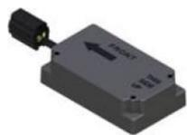
"LEVEL" SENSING UNIT - ELECTRONIC - POTTED The sensing unit has an accuracy tolerance of  $\pm$  5.4 inches front to rear and  $\pm$  1 inch side to side on a 36 foot vehicle. Typical leveling results will be better.
