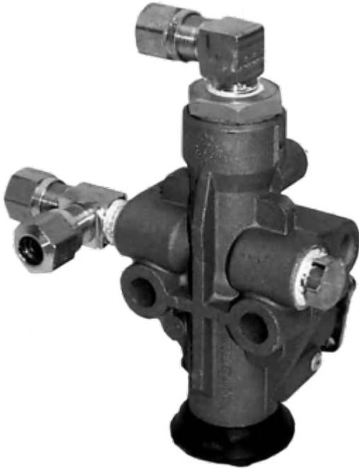
On coaches equipped with mechanical ride height valves, the typical setup is one valve on the front axle and two on the rear axle. The Valve is mounted to the frame and has a small bar connected to the suspension. When the suspension moves up and down the ride height valve's function is to add or dump air from the air bags such that proper ride height is maintained.
