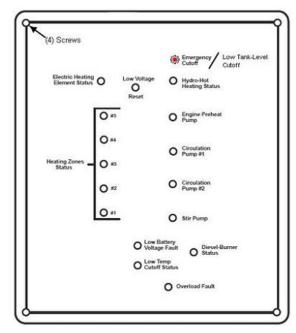
The light next to Emergency Cutoff / Low Tank Level Cut Off should be illuminated indicating low coolant.
