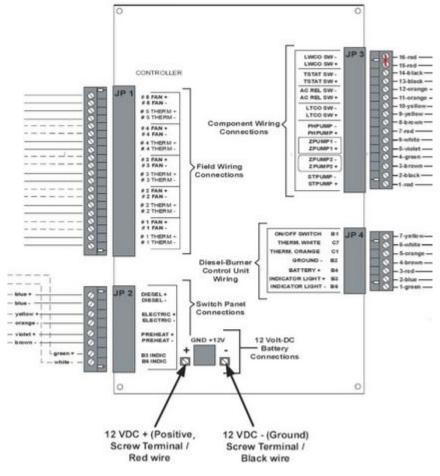
On the plug on the upper right hand corner on JP3, remove the wire # 15 and #16, (Says LWCO SW– to LWCO SW+ on the circuit board). Install a jumper wire from the terminal on the plug where wire 15 and 16 were removed. A paper clip works great!
