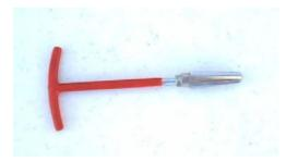
These tools are available from Lowe's, Home Depot and others. The difficulty that I had in using this tool was to get it to 'bite' into the interior of the fitting so that it could be unscrewed. Be prepared to hammer it in to get it to engage. You will need a wrench on the nut or pliers to give you additional turning force to get the fitting out. You cannot get enough leverage by using the 'T' handle.
