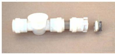
This is a pretty good picture of what the infamous drain valve looks like. I broke the threaded portion (on the right) off when I was attempting to remove the pex pipe. I suspect that it was already cracked, because it was leaking.
