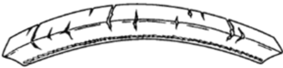
Cracked Or Split
