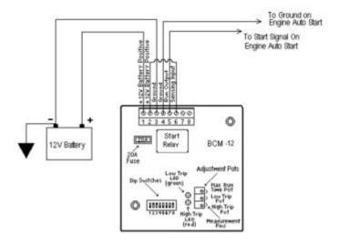
"Potentiometer" is abbreviated as "potî" throughout. To increase a pot's setting, turn it clockwise; to decrease it, counter-clockwise. These Pots are 25 turns nominal, therefore turn pots fully 25 turns to ensure that you are at either the minimum or maximum setting. The rear of the BCM unit contains three adjustable pots, and an eight position DIP switch, only 3 switches are implemented on this unit.
