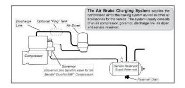
When the temperature of the compressed air that enters the <u>air dryer</u> is within the normal range, the air dryer can remove most of the charging system moisture. If the temperature of the compressed air is above the normal range, oil — as oil-vapor — is able to pass through the air dryer and into the air system. Larger diameter discharge lines and/or longer discharge line lengths can help reduce the temperature.
