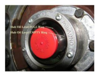
Parked on a level surface (side to side), if you are not then one side will look over full and the other side low. The oil level should be at the inner ring (below the plug), that is the full mark. Don't overfill or the oil will get slung out, don't under fill as there is not much oil protecting the bearings.
