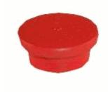
As the plug ages, it will get harder. When this happens the plug can leak around the outer edges. They also are easy to turn/spin by hand. A new plug is not as easy to turn. If you are seeing oil streaking only on the front of the wheel, then new plugs bay be in order.
