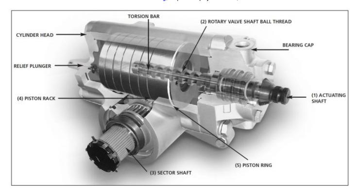
Follow the Vehicle manufacturer's recommendation for how often the steering system fluid and filter should be changed. At a minimum, this maintenance should be performed every year or every 100,000 miles, whichever comes first.
