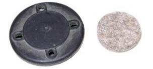
The OEM rubber covers for the ride height valves, deteriorate and fall off over time. Their purpose is to prevent dirt and contamination from entering the breather holes on the valves. They also provide some level of "muffler" to the outlet air. New covers are available for replacement, look for
