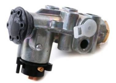
On coaches equipped with mechanical ride height valves, the typical setup is one valve on the front axle and two on the rear axle. The Valve is mounted to the frame and has a small bar connected to the suspension. When the suspension moves up and down the ride height valve's function is to add or dump air from the air bags such that proper ride height is maintained.
