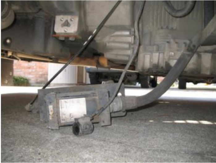
Bracket and Solenoid pieces dragging under coach. Also shows location of bracket attachment location above
