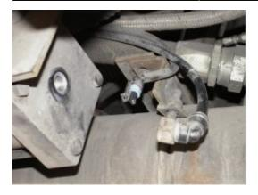
Then remove valve from retarder accumulator. Hardest part was cleaning old pipe compound from hardware threads.
