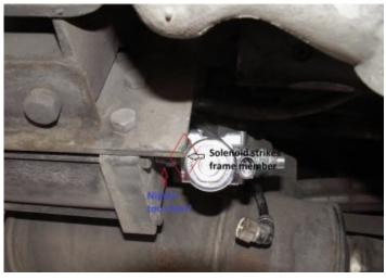
The solenoid on the new assembly is a little wider than on the old one Part #29522717. As a result, reusing the old nipple did not work. I had to get something longer. Found a 3/8" x 2" nipple at the local auto parts store, which worked fine.
