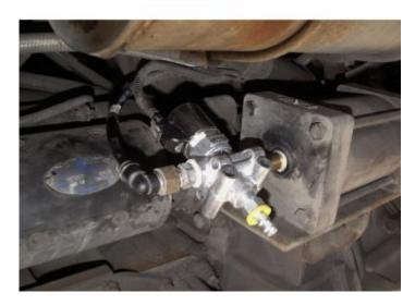
I used a TFE thread sealer. Tested for leaks with soapy solution; none found. Now we just have to confirm normal operation of the retarder on our next trip in a couple weeks.
