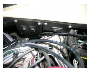
The most common location for the ABS diagnostic switch is under the dashboard cowl. Here you will typically find two (2) Momentary Switches
