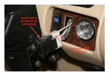
The Boost Switch has a tiny bulb that can burn out. That does not mean the Boost switch is not working. It simply means if you are having problems and are not sure, you need to have it checked. It could be just a burned out bulb.
