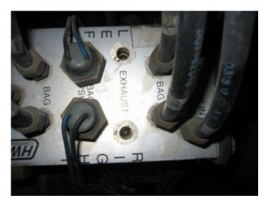
Any ride or leveling functions that require "releasing" air from the system can potentially be fouled by mud dauber nests. They like to plug up the exhaust ports on the front / rear six packs. Here are a pictures of the front pack on our coach, its those exhaust ports that will need to be cleared. Raise the coach, block it with safety blocks so you can safely go under, and clear the ports with a small screwdriver.
