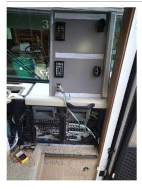
The right side of the dash in front of the passenger. The heat ducts come off easily so you can move the cover up onto the top of the dash. To take the top (horizontal portion off, I think you must remove the grab handle and then it is Velcro. I have not done this.
