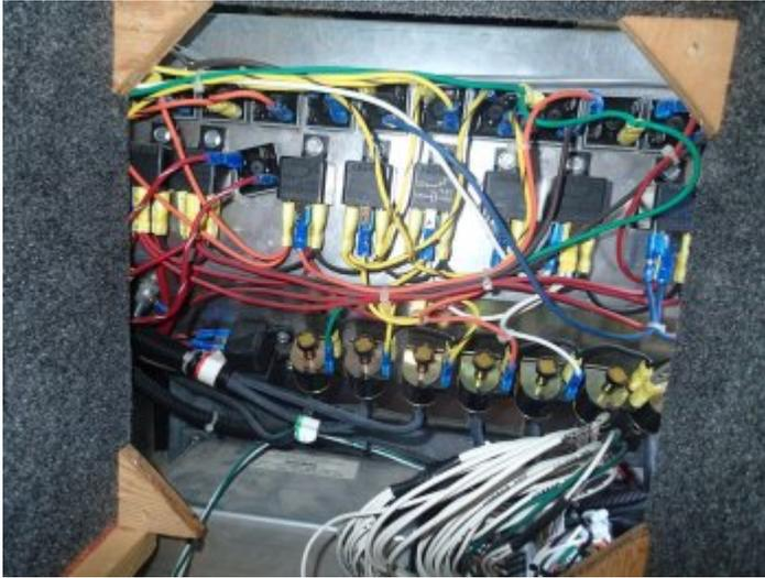
Looking into the center storage compartment. The back and bottom panels are held in with small screws. This is the top of the back of the compartment showing dash HVAC relays and vacuum control solenoids for the duct flaps.
