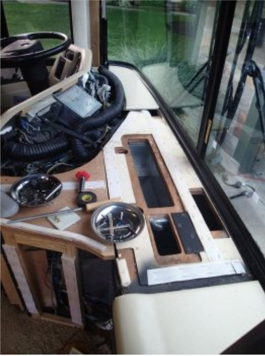
The top of the dash. The two top pieces are held on with Velcro. The cover on the back of the instrument cluster is just a push fit around the edges -no Velcro or screws.
