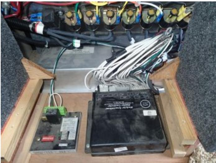
Looking down at the floor of the center compartment. In the back is the Javalina box, on the left is the controller for the Generator autostart and on the right is the Smart Wheel box.
