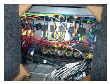
Looking into the center storage compartment. The back and bottom panels are held in with small screws. This is the top of the back of the compartment showing dash HVAC relays and vacuum control solenoids for the duct flaps.
