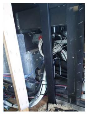
The corner between the right panel and the right side of the center console. The sheet metal box holds the blower fan and cool/heat cores.
