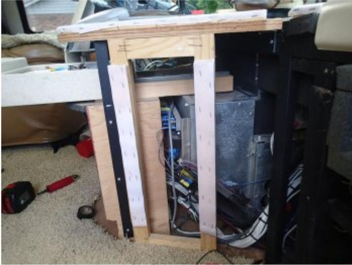
The right side of the center part of the console. It has screws on the bottom and Velcro on the top.
