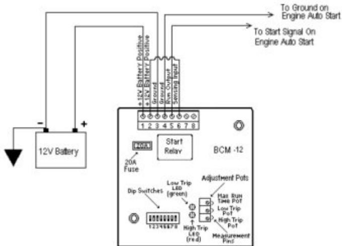
"Potentiometer" is abbreviated as "pot" throughout. To increase a pot's setting, turn it clockwise; to decrease it, counter-clockwise. These Pots are 25 turns nominal, therefore turn pots fully 25 turns to ensure that you are at either the minimum or maximum setting. The rear of the BCM unit contains three adjustable pots, and an eight position DIP switch, only 3 switches are implemented on this unit.
