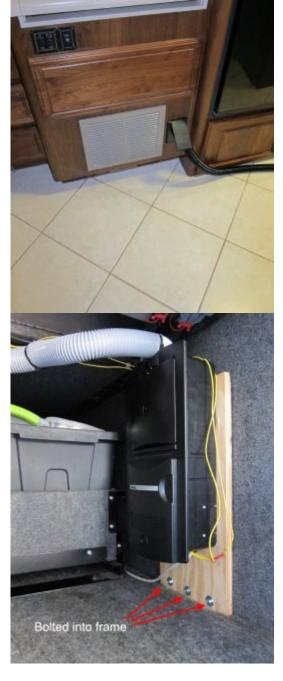
saw to cut through the floor below the galley drawers (cut from below). The floor has about 1/2" plywood on top with about 2" of blue foam and then a thin plastic layer on the bottom. No problem to cut the hole. Running the hose was no problem either (secured with wire ties). In addition to the hose, I had to run two wires (16g) to the plug-in. These turn the vacuum on when the hose is plugged in.
