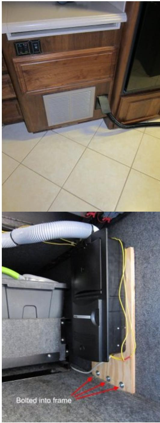
I installed the unit in the back half of our main storage bay. From there it took about 16 feet of 2" hose (purchased from Intervac) to get to the location for the vacuum hose plug-in located in the galley (see photo). I used a 2.5" hole
