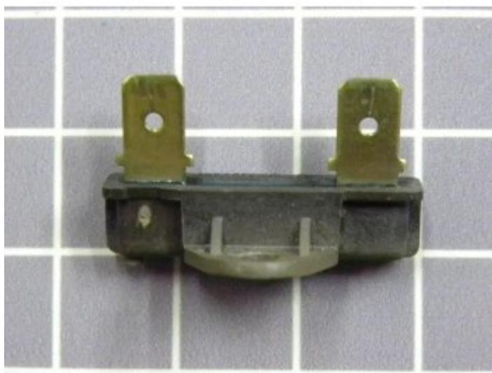
The Splendide fusible link (P/N 186240099) is a required safety device by Underwriters Laboratories. It is designed to sense an overheat situation in the dryer assembly and break the circuit in the event of overheating that cannot be controlled by the thermostat. Typically this is located on the top of the drum (under the top white sheet metal cover). If that fuse blows the heating element stops heating, but everything else still works. On some units this is a reset-able fuse.
