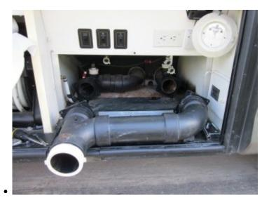
Once the panels are removed, the valves can be accessed. The dump valves are secured in place with 4 bolts (11mm socket). The pull cable "holder" also has an additional 4 screws each to remove. Once all the bolts are removed, the front piping assembly comes right off.
