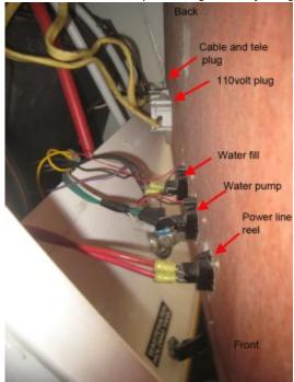
Remove top panel (three screws). This panel has three switches (at least on a 2003 coach) plus a 110v plug, and a plug for cable TV and a phone line. The switch wires are easy to remove and the rest can be removed without a lot of effort. To get this panel out you may need to remove the faucet spout and the hot water handle. The panel can pivot at the right back corner. Pull the left corner out and then once the faucet is cleared, it can be removed.
