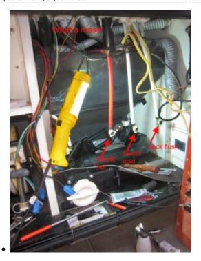
Remove the bottom panel (four screws on the bottom). It also has connections to the faucet and the black tank flush. Once everything is disconnected, the panel can be pulled up and removed. The area around the sewer outlet is rubber with a split on the bottom. This panel is a pain to take out, but you can not reach the rear bolts on the valves without taking it out.
