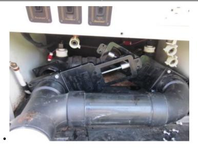
Reverse the valve disassemble process. One important note is that bolts that go through the full stack of flange + cable pull holder are longer bolts. What you get in the replacement package will not work for those 4 locations, so you have to reuse what you have or buy new.
