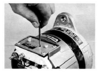
4. Turn the screwdriver clockwise to raise the voltage, counterclockwise to lower the voltage. Set the voltage between 14.0 and 14.2 volts (28.0 to 28.4 volts for 24-volt units).
