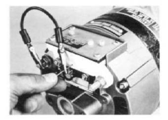
Leece-Neville alternators are equipped with one of two regulators. The Fully Adjustable Regulator has a flat cover plate. The Three Step Regulator has a finned, curved cover plate. Use the following test procedure that is appropriate for you regulator type.
