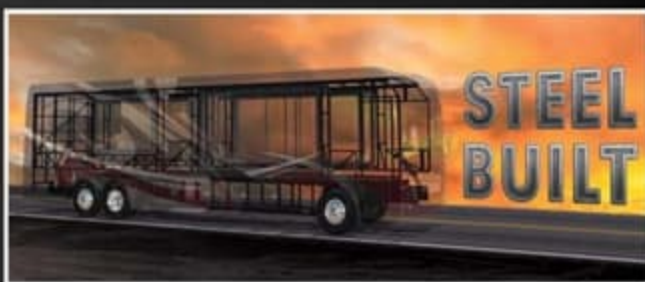
Steel construction instead of aluminum
