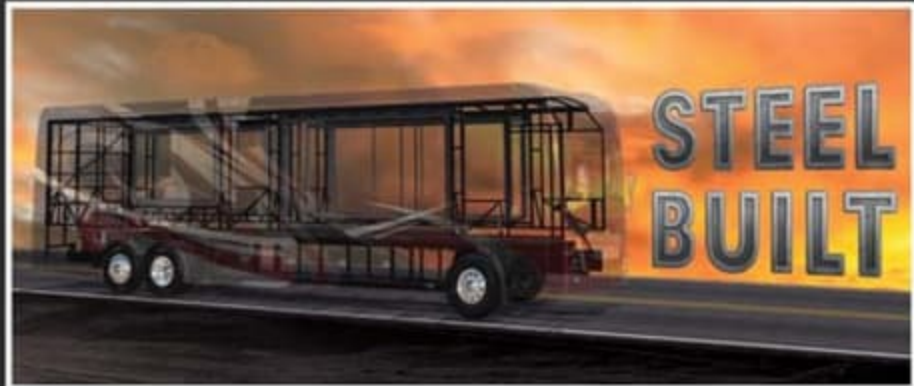
Steel construction instead of aluminum
