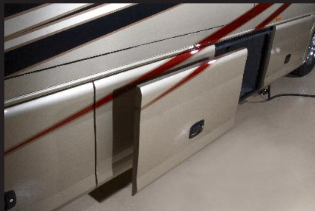
Horizontal parallel storage door for easy access to storage bay when slide room is extended.
