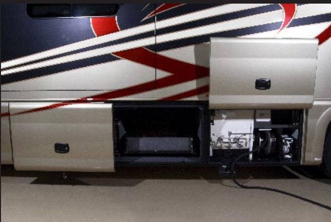
Horizontal parallel storage doors below slide rooms. Vertical storage doors in other locations. Standard on Phenix, Nimbus SE & CE, optional on Nimbus XT.
