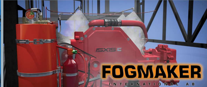
Fire Suppression System for the Engine
