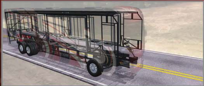
Steel construction instead of aluminum
