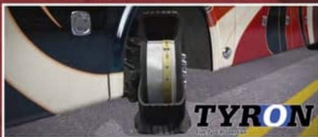
TYRON's® Bead-Lock Wheel Safety Bands
