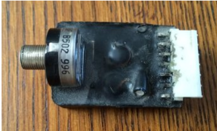
Old SGM Dash Air Temp Switch with Broken Stem
