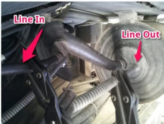
When I put my finger on the vacuum port, the pump shuts off immediately. Also, when I pinch off the vacuum tube into this can (see photo), pump shuts off, but when I pinch the tube "out", it keeps running.
