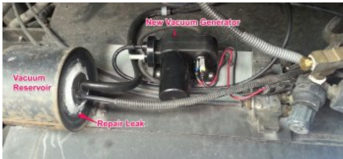
Vacuum Generator in and Reservoir repaired
