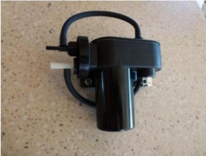
Our vacuum generator started leaking air a couple days ago inside it's little black box (located on passenger side of generator enclosure). It would drain the main air tanks in about 30 minutes. I talked to Bob at Foretravel and he said parts are no longer available for this, but they have a solution. They are sending me parts for about \$265.
