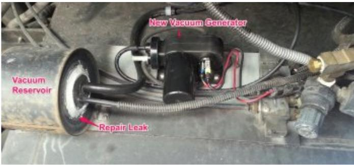
Vacuum Generator in and Reservoir repaired
