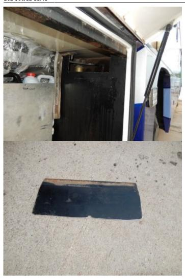
Our step has an OEM house battery disconnect rotary switch, with a pair of #2 cables connected to the switch, located in the cut-out space. We never used this switch, so we ran a short jumper between the bay mounted breakers on the other end of the cables, removing power from the cables. We removed step switch and moved these heavy cables out of the way.
