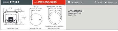
For the **Lifting Tag Axle**, these are the ones that hold downward pressure
