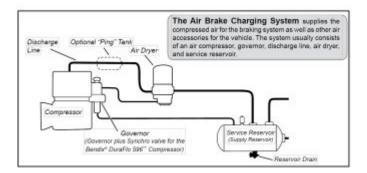
When the temperature of the compressed air that enters the air dryer is within the normal range, the air dryer can remove most of the charging system moisture. If the temperature of the compressed air is above the normal range, oil — as oil-vapor — is able to pass through the air dryer and into the air system. Larger diameter discharge lines and/or longer discharge line lengths can help reduce the temperature.
