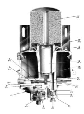
The Air Dryer is a desiccant type dryer that effectively removes moisture, oil and contaminants from the compressed air system. This reduces the risk of freezing or corrosion of the components in the air system. When compressor cut-out is reached, dry air is allowed to flow back to regenerate the desiccant bed.
