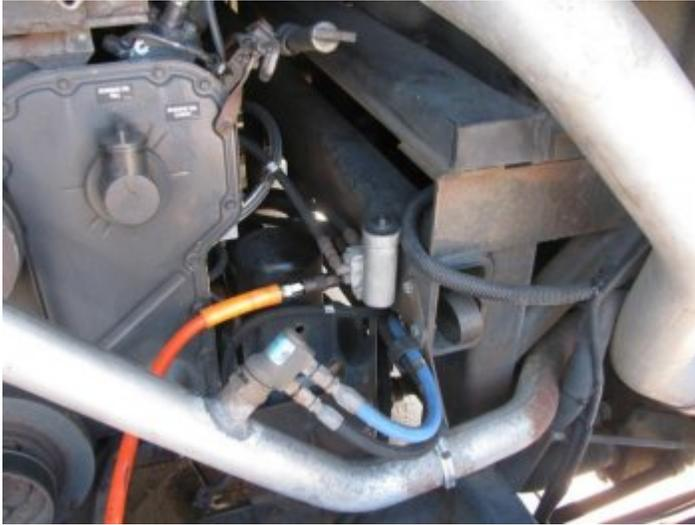
I keep a rubber plug in the Governor-installed, quick disconnect air fitting , to keep dust and particles out, when not using an air hose.
