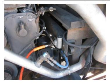
I keep a rubber plug in the Governor-installed, quick disconnect air fitting , to keep dust and particles out, when not using an air hose.
