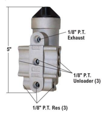
The Governor is most often referred to as the D-2 Governor. It is made by Bendix but there are many brand names that make D-2 Governors. The D-2 is very versatile, capable of many different setups with lot of ports / positions/ options. Because of the different setups possible, it is VERY important to match the holes with the old unit or you can create a not operating system.
