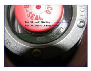
The hubs use 85W-140 gear oil, you can find it anywhere including Walmart. Just remove your front hub caps / "top hats" (pull off the decorative lug covers and the rest will come right off). Once done you will see a red cap, its a rubber plug and will pull right out. Add in the gear oil until you are at the full line and put the plug back in.
