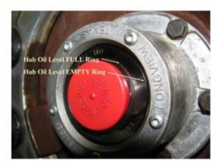
Parked on a level surface (side to side), if you are not then one side will look over full and the other side low. The oil level should be at the inner ring (below the plug), that is the full mark. Don't overfill or the oil will get slung out, don't under fill as there is not much oil protecting the bearings.
