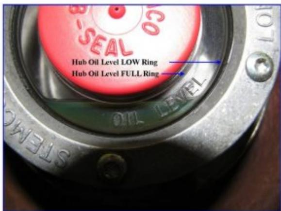
The hubs use 85W-140 gear oil, you can find it anywhere including Walmart. Just remove your front hub caps / "top hats" (pull off the decorative lug covers and the rest will come right off). Once done you will see a red cap, its a rubber plug and will pull right out. Add in the gear oil until you are at the full line and put the plug back in.
