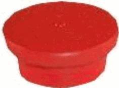
As the plug ages, it will get harder. When this happens the plug can leak around the outer edges. They also are easy to turn/spin by hand. A new plug is not as easy to turn. If you are seeing oil streaking only on the front of the wheel, then new plugs may be in order.
