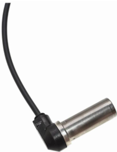
**Pickup** — The pickup is commonly called “the sensor.” It contains a wire coil/magnet assembly, which generates pulses of electricity as the teeth of the exciter pass in front of it. The ECU uses the pulses to determine wheel speeds and rates of acceleration/deceleration. The strength of these electrical pulses decreases rapidly with slight increases in the gap between the pickup and the exciter.
