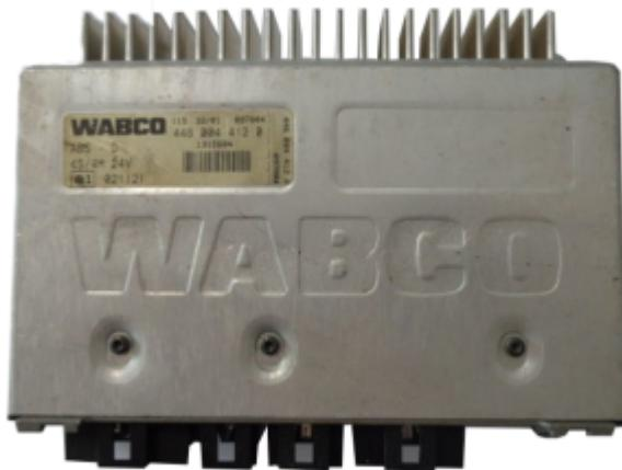
The ECU processes all ABS information and signal functions. It receives and interprets voltage pulses generated by the sensor pickup as the exciter teeth pass by, and uses this information to determine:
