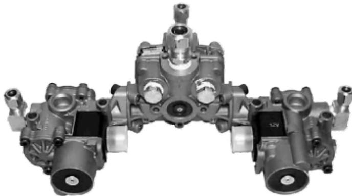
ABS Modulator Valves regulate the air pressure to the brakes during ABS action. When not receiving commands from the ECU, the modulator valve allows air to flow freely and has no effect on the brake pressure. The ECU commands the modulator valve to either:
