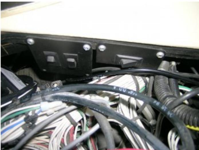
The most common location for the ABS diagnostic switch is under the dashboard cowl. Here you will typically find two (2) Momentary Switches
