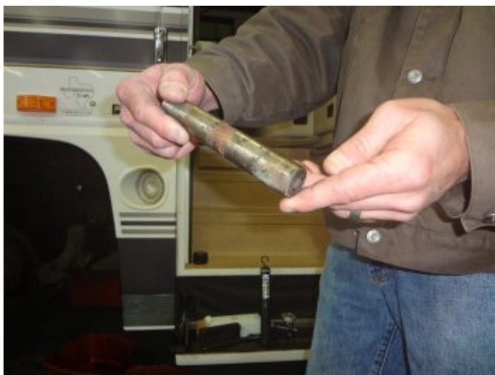
Corroded Slide Pin
