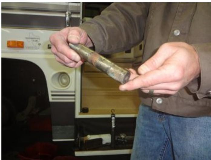
Corroded Slide Pin
