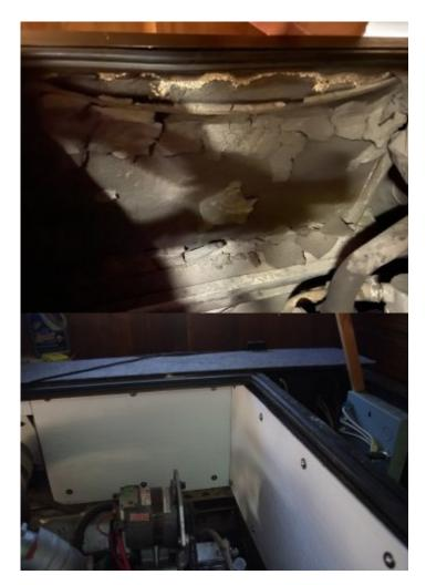
Over time the engine compartment insulation degrades and needs to be replace or recovered. Here are several ways that have been used.
