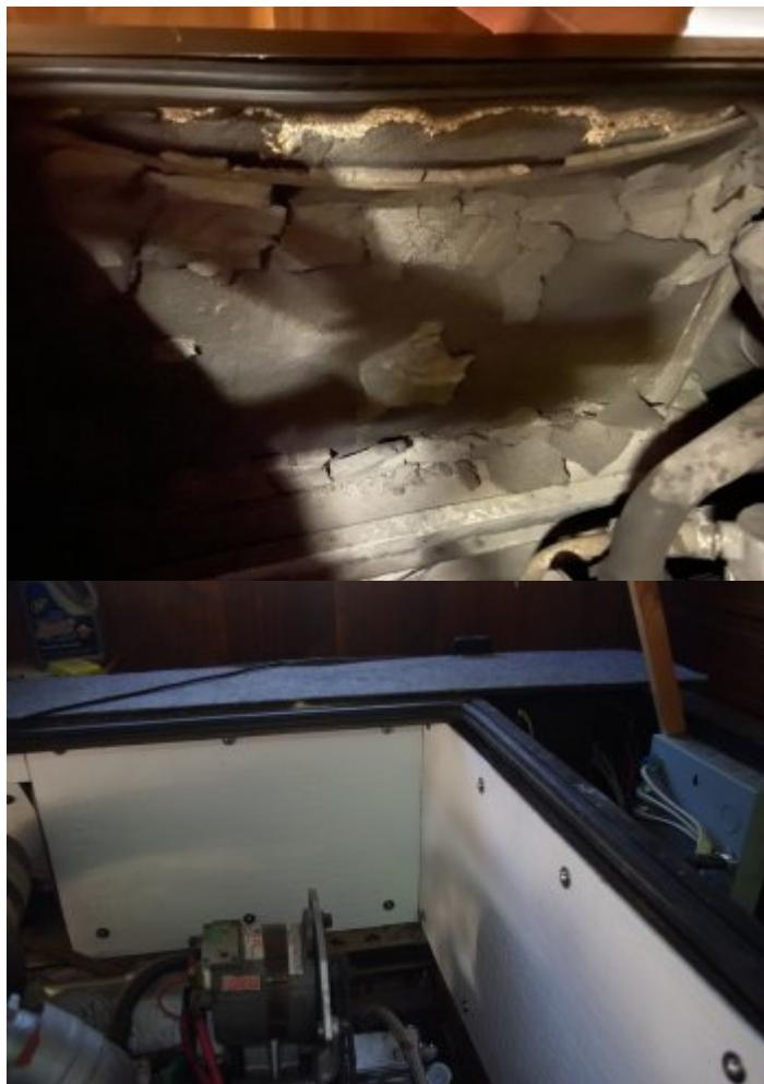
Over time the engine compartment insulation degrades and needs to be replace or recovered. Here are several ways that have been used.
