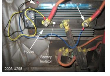
There are several devices that allow this on the market. One of the most popular is Trik-L-Start (no longer accepting orders) Simply connect one wire to each side of boost solenoid or isolator and a third wire to ground. This device
