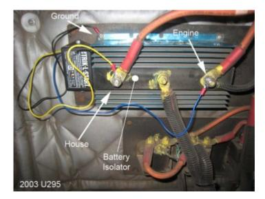
There are several devices that allow this on the market. One of the most popular is Trik-L-Start (no longer accepting orders) Simply connect one wire to each side of boost solenoid or isolator and a third wire to ground. This device
