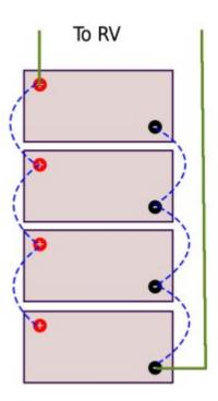
All that has changed in this this method is that the main feeds to the rest of the installation are taken from diagonally opposite posts.
