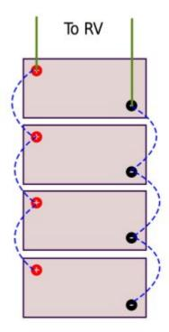
In this (not recommended) method, the connections to the main installation are all taken from one end.
