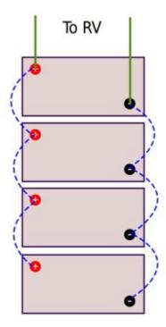
In this (not recommended) method, the connections to the main installation are all taken from one end.
