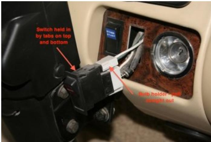
The Boost Switch has a tiny bulb that can burn out. That does not mean the Boost switch is not working. It simply means if you are having problems and are not sure, you need to have it checked. It could be just a burned out bulb.
