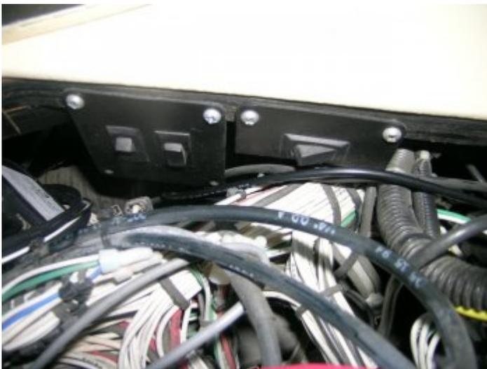
The most common location for the diagnostic switch is under the dashboard cowl. Here you will typically find two (2) Momentary Switches, the normal arrangement is:
