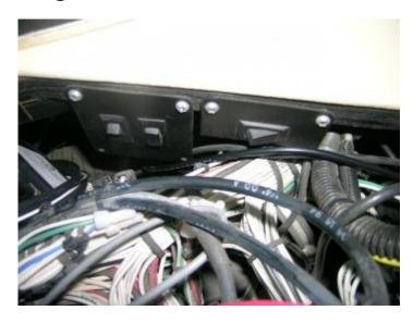
The most common location for the diagnostic switch is under the dashboard cowl. Here you will typically find two (2) Momentary Switches, the normal arrangement is:
