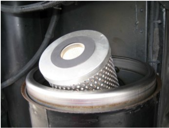
Last of three filters on the way to sitting on top of other filters. Each filter slips over center post
