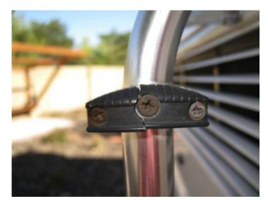
Broken step mounting before replacement. Very dangerous to use ladder with broken or cracked ends. Care must be taken to examine each step end and those creaks when climbing rear ladder should be taken seriously.
