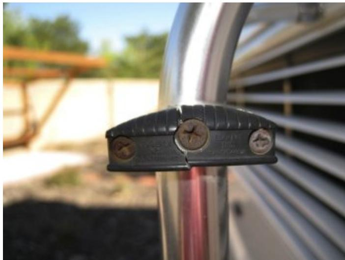
Broken step mounting before replacement. Very dangerous to use ladder with broken or cracked ends. Care must be taken to examine each step end and those creaks when climbing rear ladder should be taken seriously.
