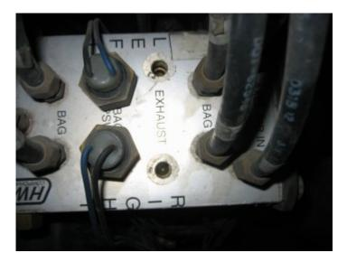
Any ride or leveling functions that require "releasing" air from the system can potentially be fouled by mud dauber nests. They like to plug up the exhaust ports on the front / rear six packs. Here are a pictures of the front pack on our coach, its those exhaust ports that will need to be cleared. Raise the coach, block it with safety blocks so you can safely go under, and clear the ports with a small screwdriver.
