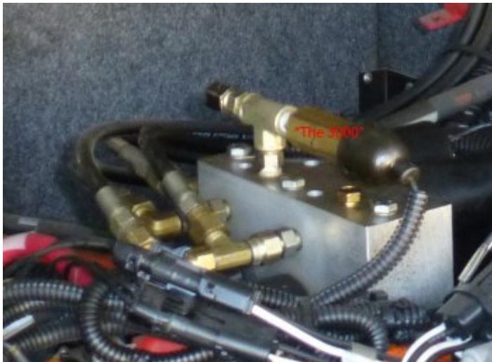
When the hydraulic pump does not stop running when a room reaches its inner or outer limit and the red panel light does not go out, and this happens for all side rooms, then its likely the high pressure switch "The 3000" is the culprit
