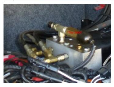
When the hydraulic pump does not stop running when a room reaches its inner or outer limit and the red panel light does not go out, and this happens for all side rooms, then its likely the high pressure switch "The 3000" is the culprit
