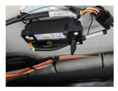
The original level sensor is located "somewhere" inside the coach, normally fastened to the floor under a cabinet / sofa. The original unit used mercury to sense when coach was not level.
