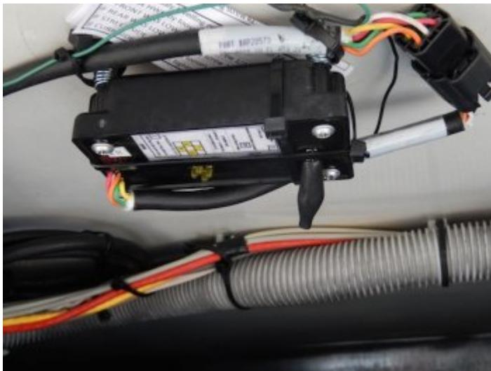
The original level sensor is located “somewhere” inside the coach, normally fastened to the floor under a cabinet / sofa. The original unit used mercury to sense when coach was not level.
