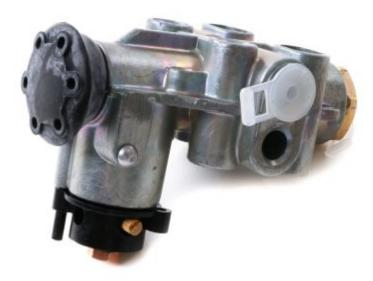
On coaches equipped with mechanical ride height valves, the typical setup is one valve on the front axle and two on the rear axle. The Valve is mounted to the frame and has a small bar connected to the suspension. When the suspension moves up and down the ride height valve's function is to add or dump air from the air bags such that proper ride height is maintained.
