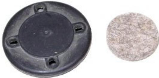
The OEM rubber covers for the ride height valves, deteriorate and fall off over time. Their purpose is to prevent dirt and contamination from entering the breather holes on the valves. They also provide some level of "muffler" to the outlet air. New covers are available for replacement, look for
